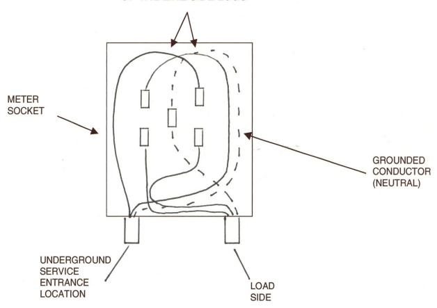
LOOPING OF CONDUCTOR AS SHOWN MINIMIZES DAMAGE TO CABLE AND STRESS ON CONNECTIONS
